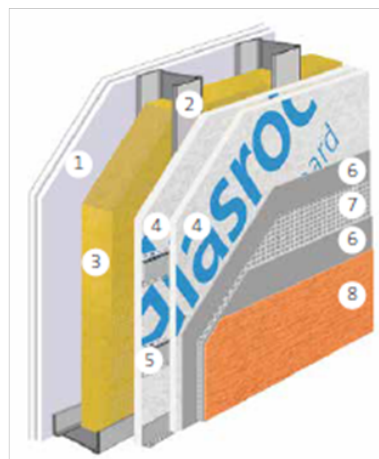
Figure A.3. Schematic representation of the External wall with Cladding system (Glasroc® X).
