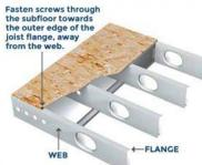
What about fasteners? Where should you place the screws in a joist? Answer: Screw the subfloor into the joist flange as far from the web as you
