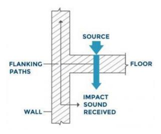
As noted in these diagrams, airborne sound and impact sound are transmitted in two ways:
